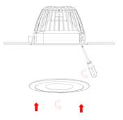
3. Put the downlight into the ceiling. Tighten the three ceiling clips by screwdriver and rotate the ring back.
